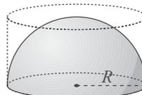
$$V_{SEMIESFERA} = \left(\frac{2}{3} V_{CILINDRO}\right)$$
